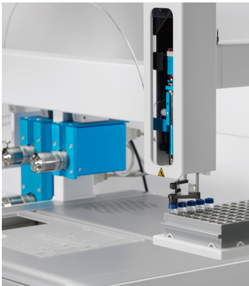
Automation of the LC-GC with a CTC-sampler
