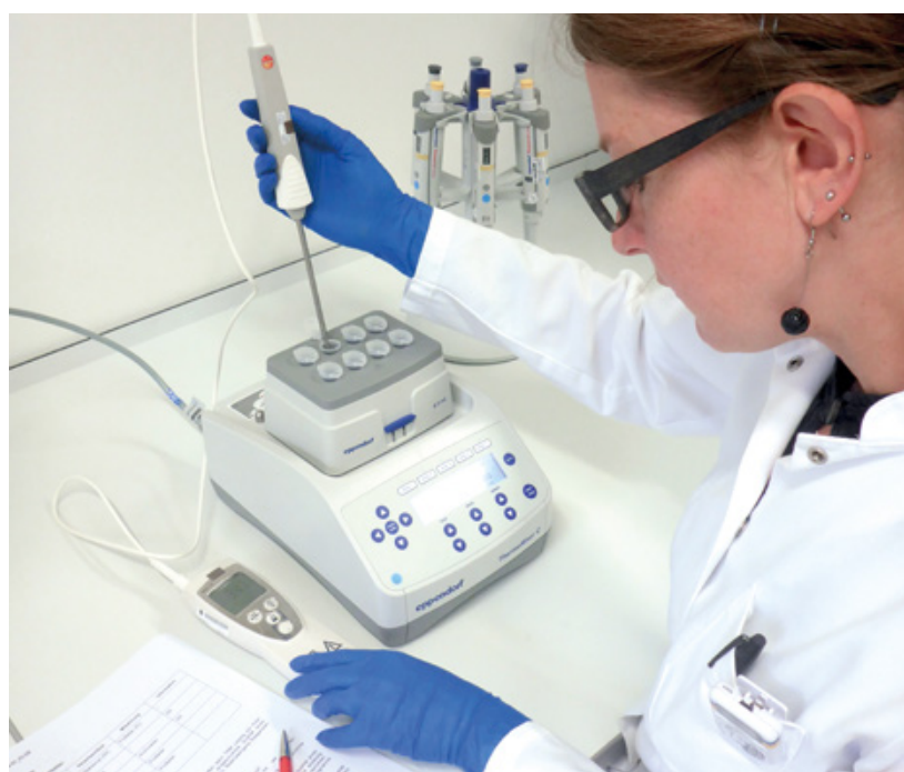
Fig. 3 Qualification of a thermocycler. Equipment used within GLP must be both calibrated and qualified.
