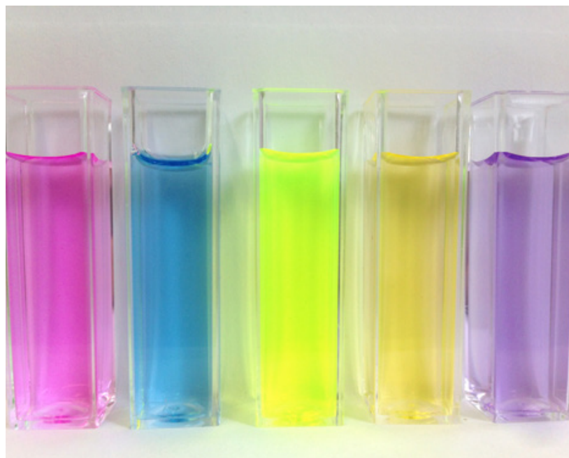
Fig. 2 Picture of ion selective nanosphere aqueous suspensions containing various chromoionophores.
